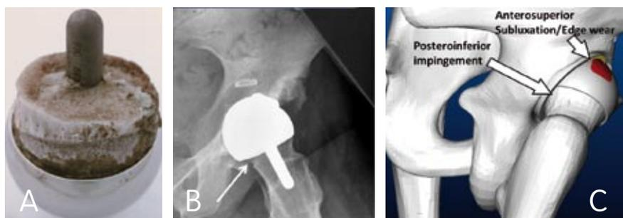
Figure 18: Showing (A) the explanted femoral component with an indentation in the posterior femoral neck from the impingement, seen radiographically (arrow in B), and shown schematically (C) along with the anterior subluxation and edge loading leading to excessive wear in Case 3
