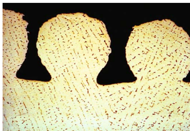
FIG. 1.67. Section through Porocast beads and cup substrate metal. Beads are integral with cup substrate metal. Carbides (dark dots) in microstructure can be seen.
