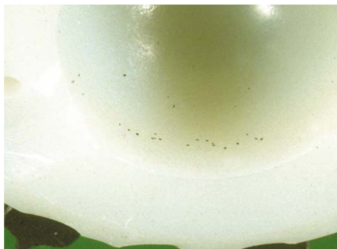
FIG. 1.66. Polyethylene liner removed at revision with embedded plasma-sprayed titanium particles. Plasma-sprayed acetabular shell was solidly fixed.
