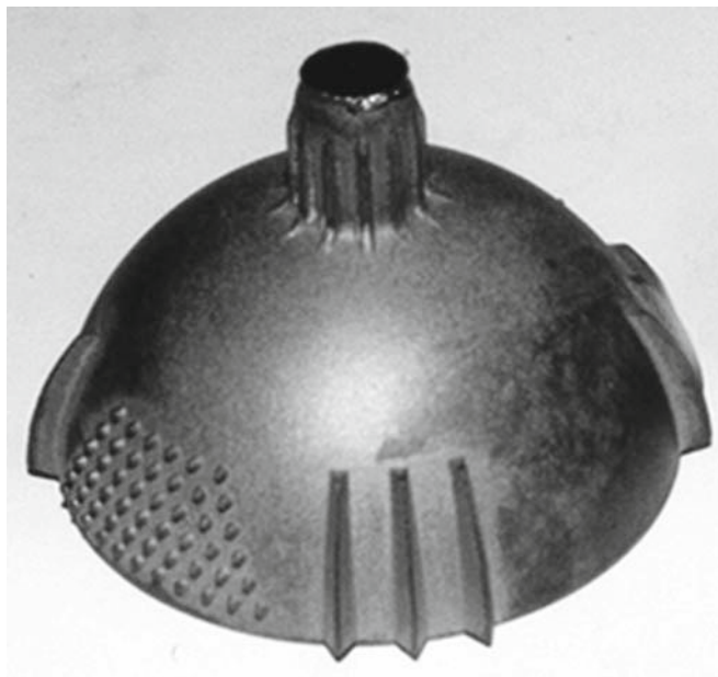
FIG. 1.52. New variety of cup before HA coating. Three of the four sets of antirotation fins can be seen.
