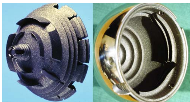
FIG. 1.34. Initial variety of cementless metal on metal resurfacing. Cup and head had porous titanium ingrowth surfaces with cobalt chrome articular surfaces. Femoral component was of a “screw-on” type.
