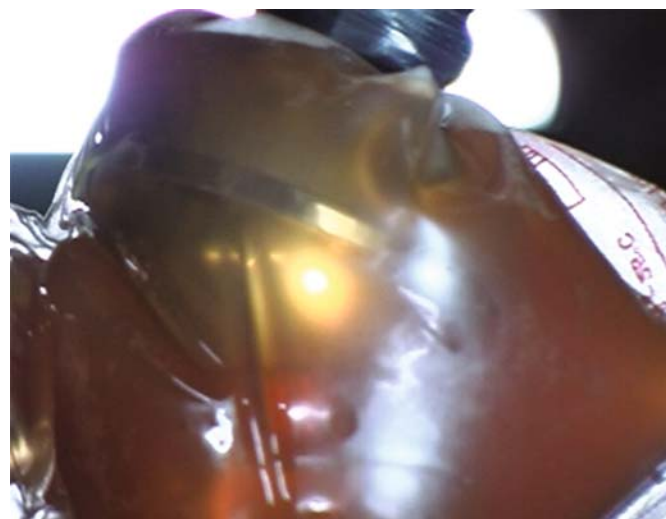
FIG. 1.28. This shows metal on metal couple with the acetabular component on top. Outside the prosthesis is a membrane containing serum and hyaluronic acid.
