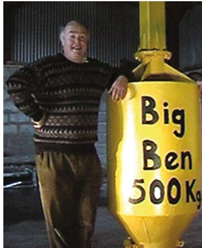
FIG. 1.25. Author standing beside 500-kg concrete-filled steel bob. This weight was necessary to give realistic high loading on prosthetic hip joints.
