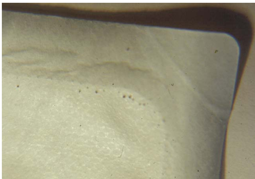
FIG. 1.65. Plasma-sprayed titanium particles in packaging box having fallen off the porous surface of an acetabular cup.
