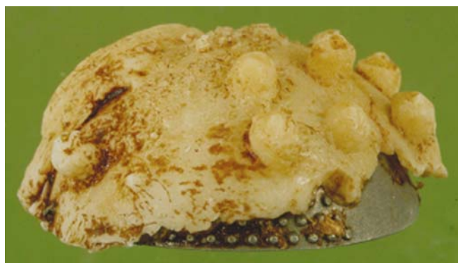
FIG. 1.44. Cemented cup removed for loosening.
