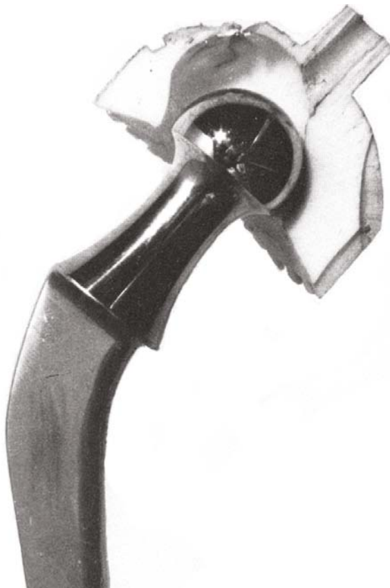
FIG. 1.24. Total wear-through of a Charnley Teflon cup after 3 years showing vertical direction of wear track. (Reproduced with permission from Springer).
