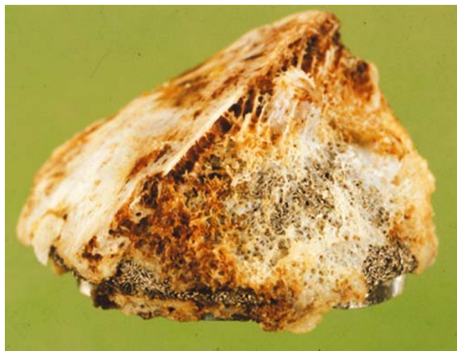
FIG. 1.30. Harris-Galante I cup shell together with osseointegrated acetabulum removed at revision surgery.
