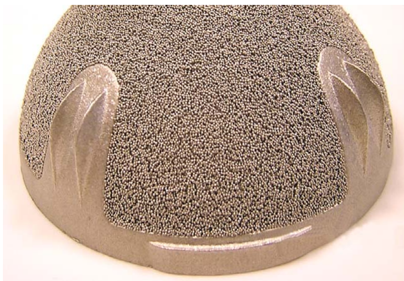
FIG. 1.64. Sintered beaded BHR cup. Because of microstructural damage of the metal, this implant was never used clinically.
