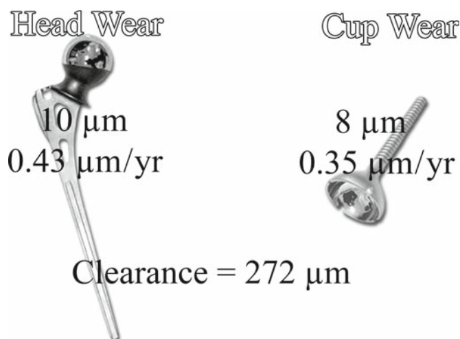
FIG. 1.14. Wear and clearance measurements of the components removed from the patient of Fig. 1.13.
