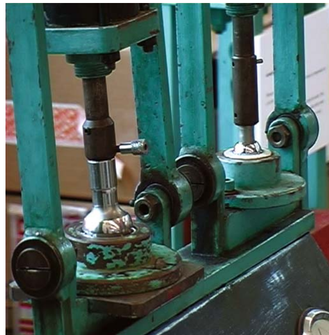
FIG. 1.23. The McKee-Farrar metal on metal couple (nearest) came to a juddering halt despite the application of human synovial fluid, and the Charnley metal on polyethylene couple (farthest) kept on swinging.
