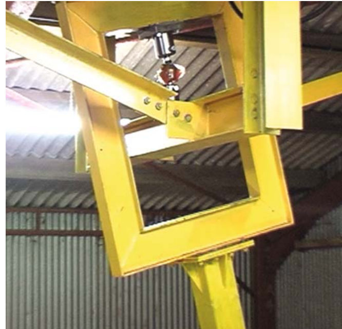
FIG. 1.27. Loading area for test hip joint prostheses high in roof space. When stationary, a hydraulic ram is attached to distract the apparatus and load a new joint for testing.
