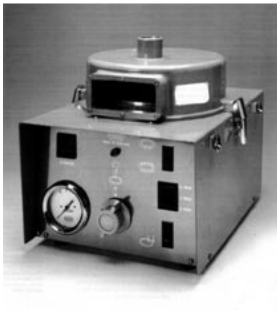
Figure 25: Casella slit sampler AIR14 used in the 1960 clean air enclosure, originally developed by the Medical Research Council. See Bourdillon et al. (1948): 15.
