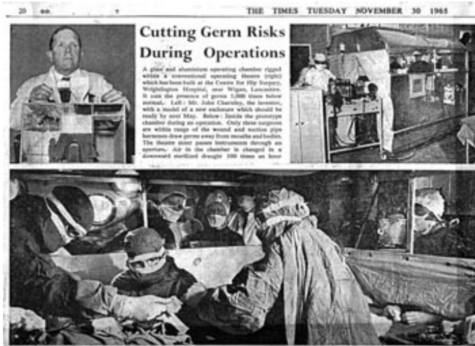
An operation in progress in "The Greenhouse." Only three surgeons go inside, aseptic operator stays outside. Cool air blows downwards—germs are forced out underneath.
