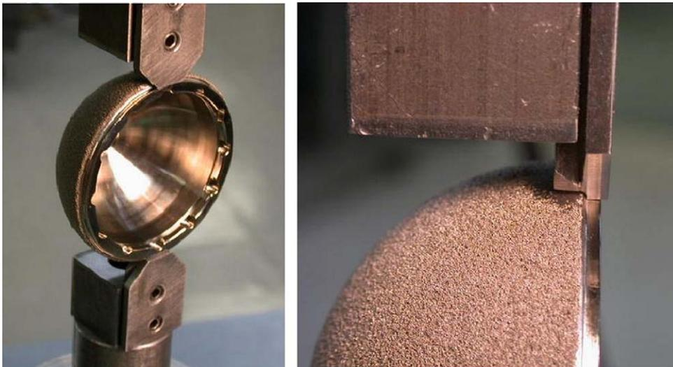
**Fig. 2.** Custom-designed load platens provided rim loading of the acetabular cup during mechanical testing.
