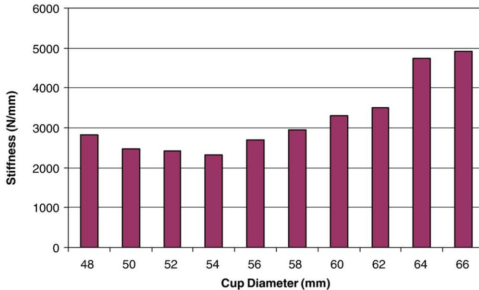
Fig. 3. Bar graph of stiffness values (mean  $\pm$  SEM) for each of the 10 acetabular cups tested.
